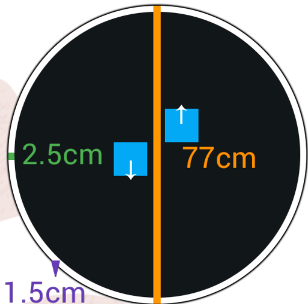
Figure 1. Diagram of the Dohyo with two blue sumobots placed antiparallel, as is prior to the start sequence. The orange line represents the center of the Dohyo and will not present on the Dohyo used during the competition.
